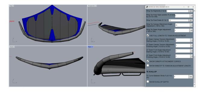
Along with these tools there is now a display option showing the original and modified canopy attachment line on the LE:
