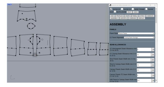
KITE - separate control for canopy panel seams at struts
